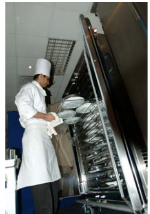
Loading a Versigen Chillogen Banqueting trolley. The trolley chills & holds meals at <5°C before heating to >70°C just before service - automatically!
