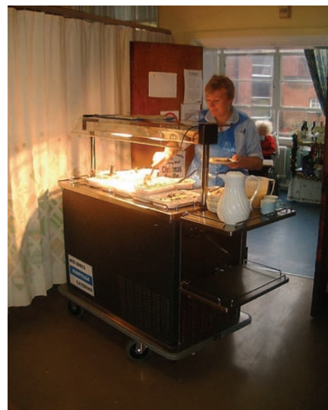
Hostess service from the Versigen - note the two end shelves, added by Versigen at the Catering Manager's request
